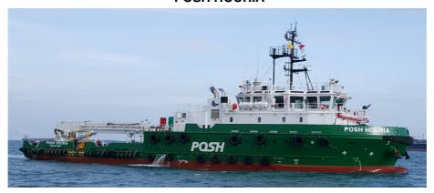
3,150 BHP / 49.4M / Utility Maintenance Vessel Call Sign: 9V5130
