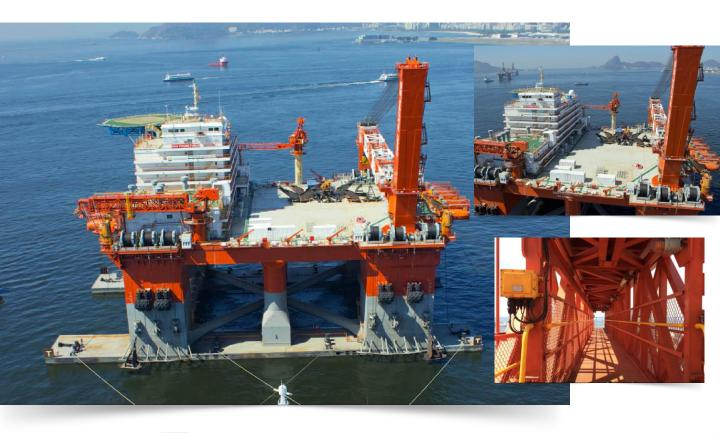
Semi submersible vessel with accommodation capacity of 500 beds and a 1100T offshore mast crane, CIMC Prometheus is suitable for your 0&G projects that includes offshore heavy construction, decommissioning, installation, modification and removal activities.
