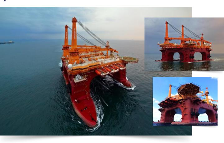
Self Propelled dynamically positioned semi submersible vessel with 2 x 1800T crane lifting capability. With 618 available beds and a tandem capability of 3600MT, CIMC Gretha is suitable for your 0&G or Offshore Renewable projects that includes offshore heavy construction, decommissioning, installation, modification and removal activities.
